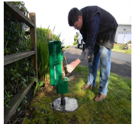
SRWD Technician takes a water sample from one of the District's many sampling stations:
